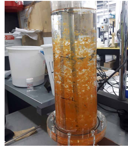
Figure 15. Flocs in the laboratory DAF column before the fine air bubbles are introduced into the column
