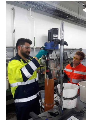
Figure 15. Flocs in the laboratory DAF column before the fine air bubbles are introduced into the column
