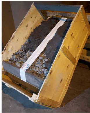
Figure 8. Installation on inclined surfaces of waste rock at two different angles. The cover recipe was applied at the top end of the inclination.
