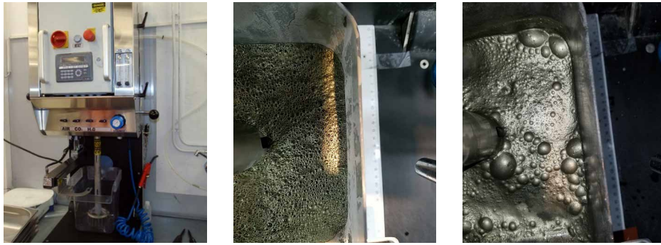
Figure 17. Outotec GTK LabCell for laboratory flotation tests (left), and concentrates (right)
