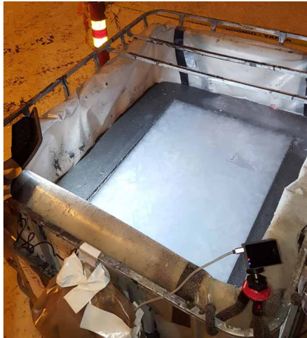
Figure 9. Horizontally installed cover on high-sulfur waste rock. The surface pool was filled with water and then exposed to the outside conditions (temperature up to -16^\circ\text{C} ) to simulate freeze-and-thaw cycles.
